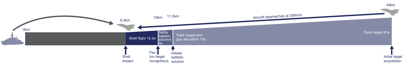
Fixed wing aircraft first target triggered burst (TTB) at 6.3km
