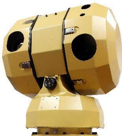
The Chess Dynamics Guardian, part of the Hawkeye Land electro-optics family, is a long range surveillance and fire control director, suitable to be fitted weapon platforms as well as for border surveillance.
