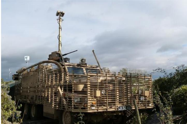
The Chess Dynamics Cobra Hawk fitted on a Mastiff. Cobra Hawk is part of the Hawkeye family of land electro-optical systems which utilise common user interfaces and modularity.
