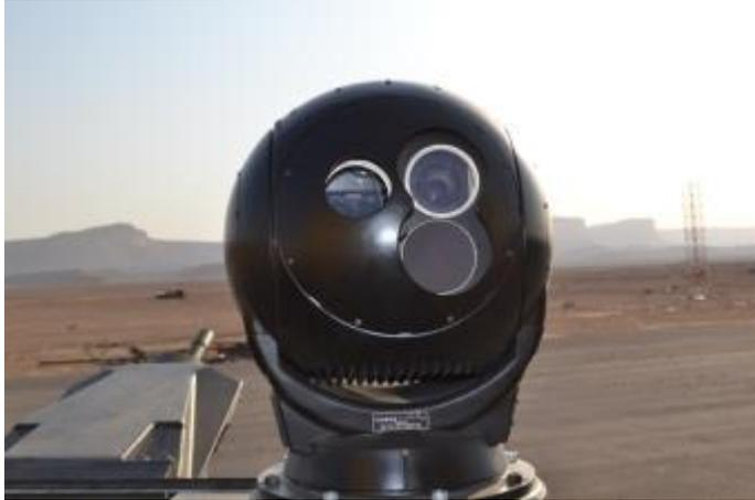
The Hawkeye Combat System is a rugged, compact EO equipment designed to meet the exacting requirements for turreted and non-turreted AFVs.
