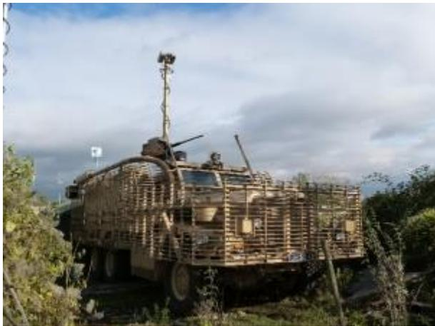
The Hawkeye Vehicle System mounted on a Mastiff. Included in the system are thermal and daylight sensors. The mast mounted system can be used on the move.
