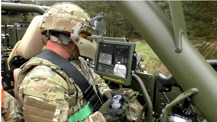
The Chess Dynamics Hawkeye Electro Optic Vehicle System uses a touch screen, icon based display with a Game Pad style controller to reduce the operator's workload.
