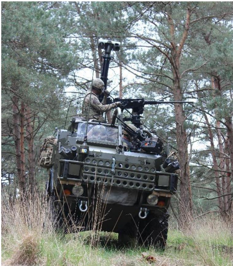
The Chess Dynamics Hawkeye, Electro Optic, Vehicle System, fitted to a Jackal recce vehicle, is an easy to use, easy to fit surveillance system which allows the operator to see out to 20km using a long range day/low light camera.
