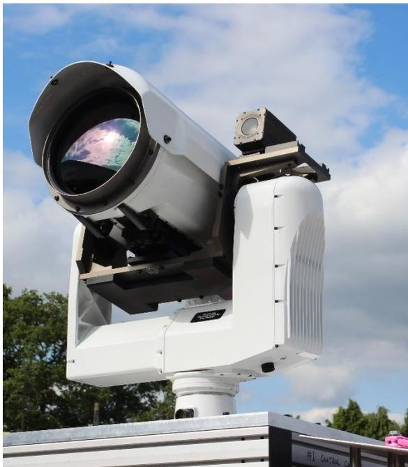
An example of the Chess Sigma LEO sensor head with Long Range Thermal Imaging and TV cameras.
